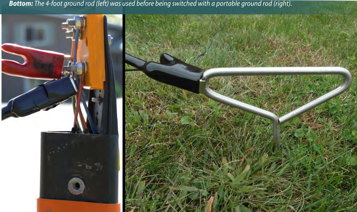
Top: Mike Parilac hooks up his transmitter to test the tracer wire viability on the job, which checks out ok. Top Right: These above ground telephone structures indicate the presence of parallel-positioned telephone duct. Bottom: The 4-foot ground rod (left) was used before being switched with a portable ground rod (right).
