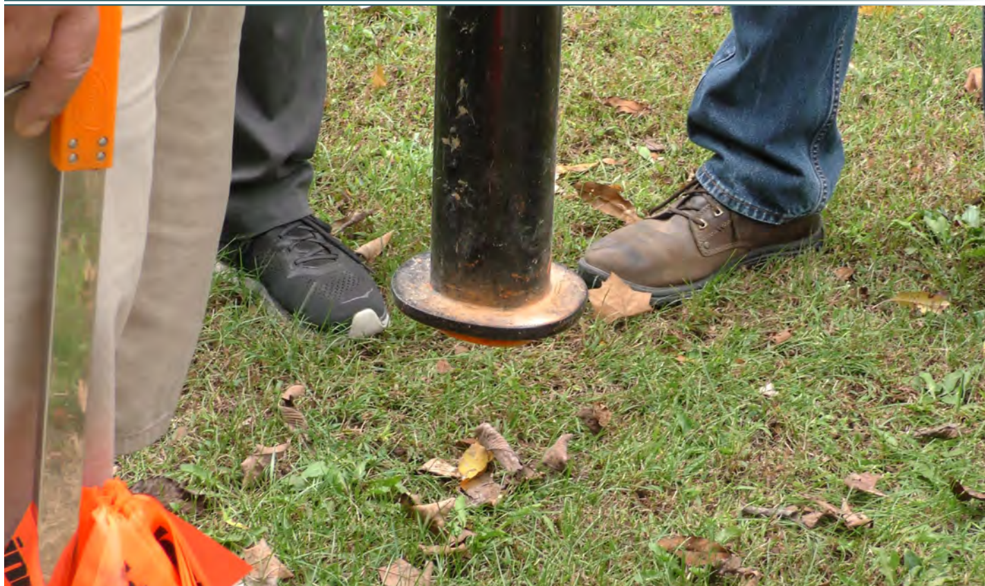
Patrick lifts the receiver to read the depth at a second elevation to validate the initial depth reading.
