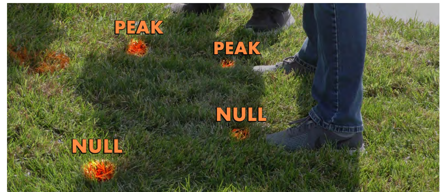
Sometimes there is too much metal in the locate area that becomes energized by the transmitter. In this case, the metal was a group of copper telephone cables running parallel with the tracer wire. After moving the transmitter to the end point and sending the signal the opposite way, and trying a lower frequency, the gap between the high peak number (right foot) and the arrows of the null reading (left foot) did shorten up quite a bit, but it was still about a foot off from lining up.
