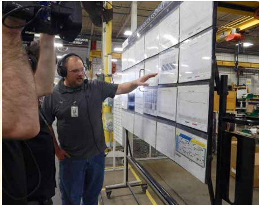
Matt shows us their factory Managing for Daily Improvement (MDI) Board where key items such as quality, safety, delivery, and cost control are continuously monitored. The 5S column contains a check list of daily tasks and tracking of any problems that may arise on the floor.
