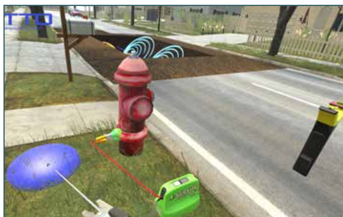
VR environment showing how to hook-up a portable transmitter and earth stake. A user is scored based on successful hook-up.
