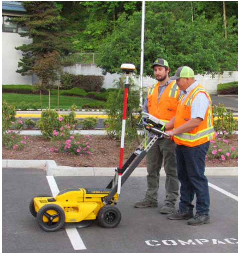
Kemp operating an IDS Opera Duo GPR locator with integrated GPS.
